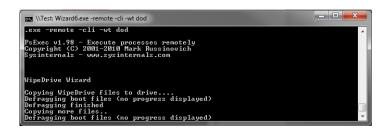
As you can see PsExec copied the WipeDrive Wizard and began installing the necessary tools to remotely run the software.
